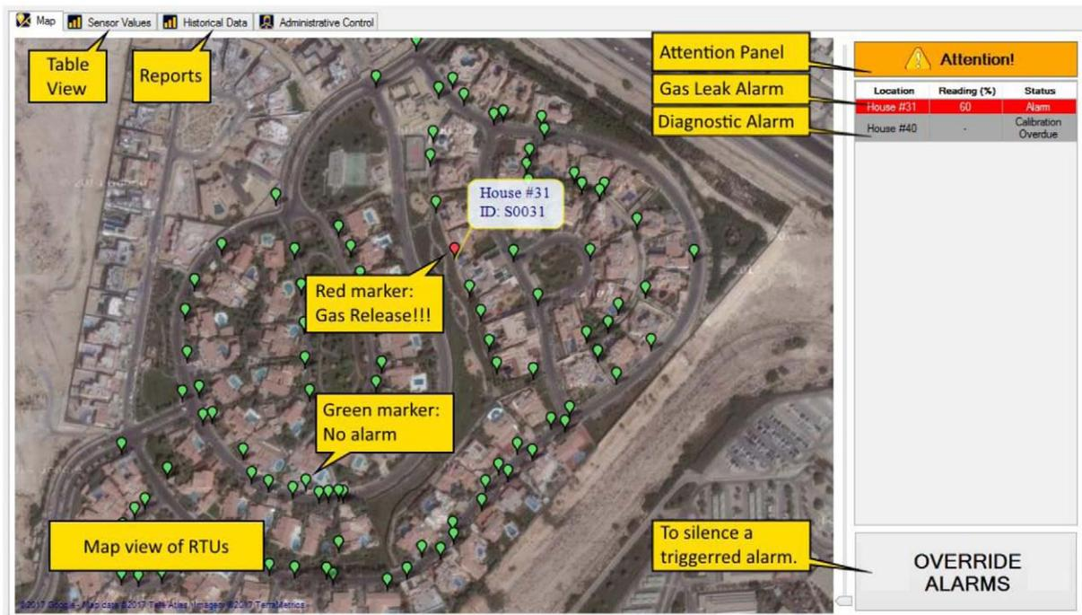
Figure 2—View of the SCADA software running on the system monitors
