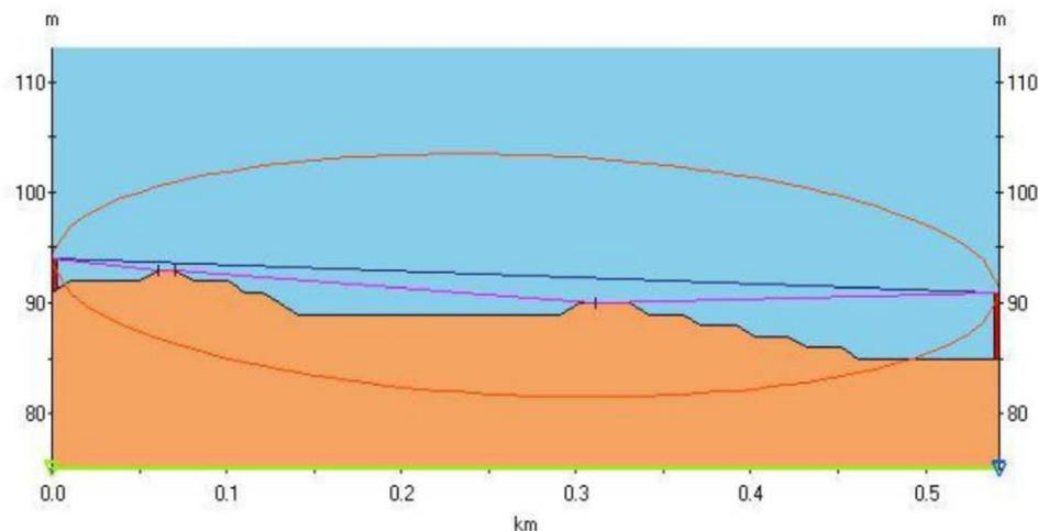
Figure 3—Sample of the link budget simulations between the controller and a RTU
