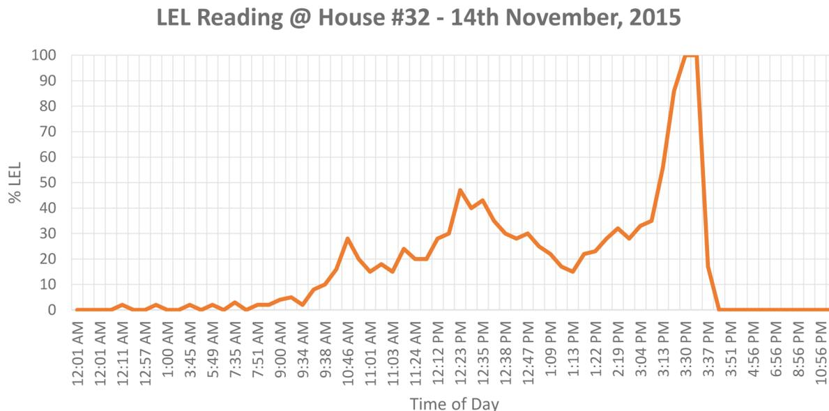
**Figure 4—Plot of the gas readings leading up to and after a gas alarm detected by the wireless gas detection system**
