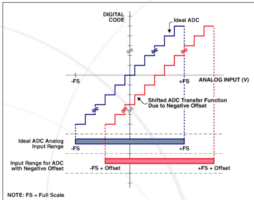
FIGURE 1: BIPOLAR OFFSET ERROR IN AN ADC
