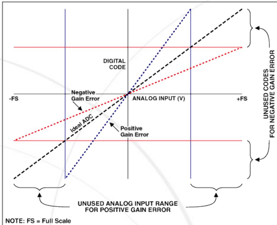
FIGURE 2: GAIN ERROR IN ADCs
