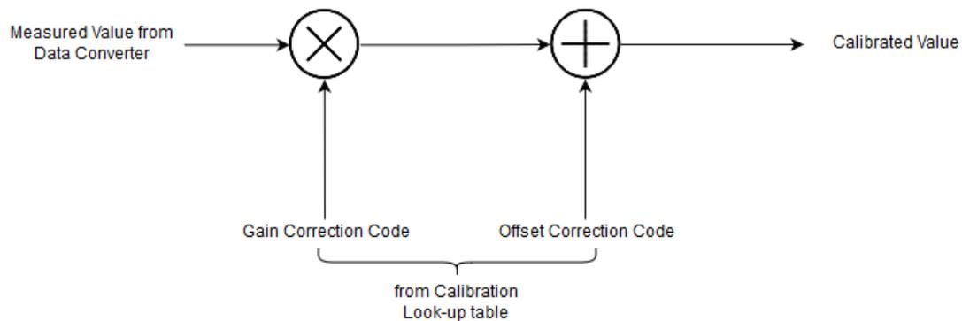
FIGURE 3: THE ARITHMETIC PROCESS TO DIGITALLY CALIBRATE OUT DATA CONVERTER ERRORS
