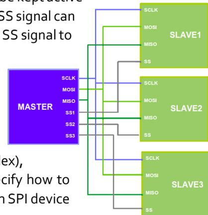
FIGURE 2: SPI BUS STRUCTURE
