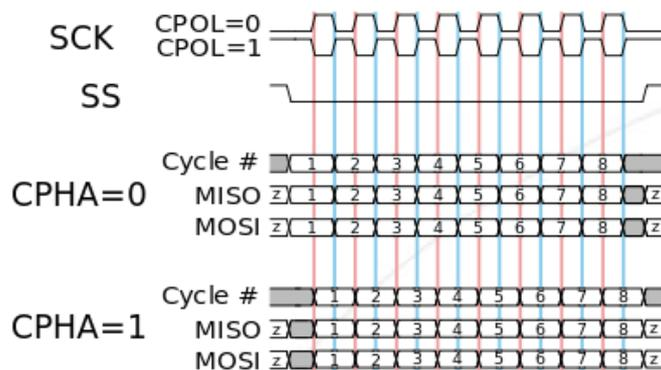
**FIGURE 3: SPI BUS TIMING**
